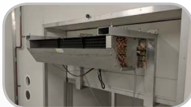
Image 3: Citimax 700 evaporator unit in thermal test chamber
