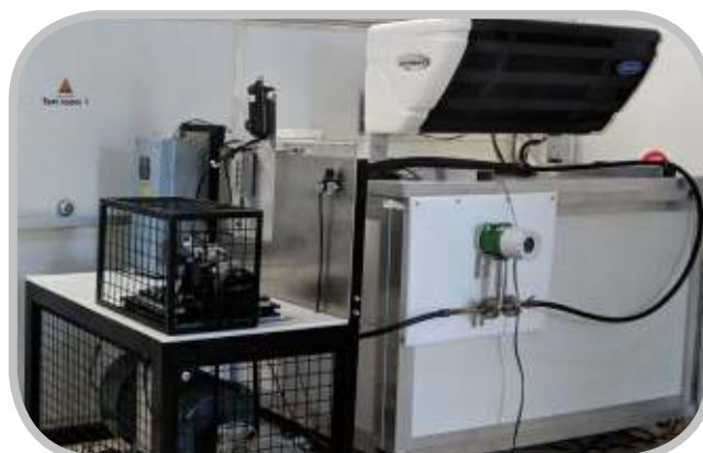
Image 2: Motor bench and Citimax 700 condenser unit in thermal test chamber
