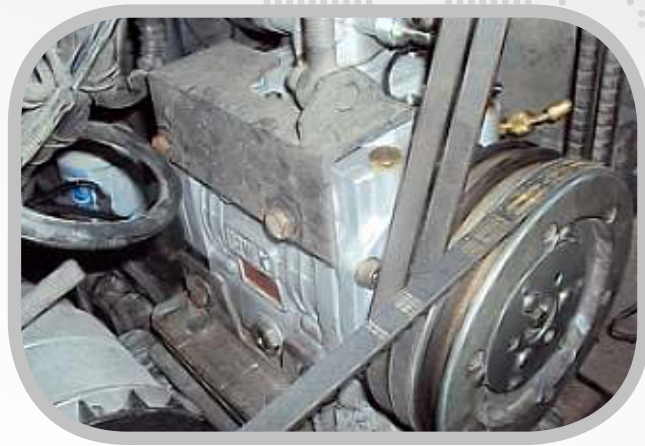
Custom compressor mount bracket and 3B clutch pulley.
