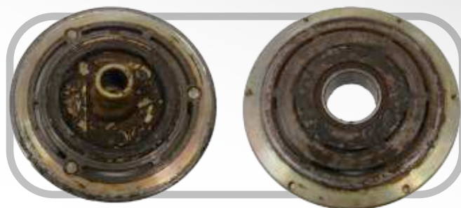
The armature was jammed against the pulley by solidified mud and grime
