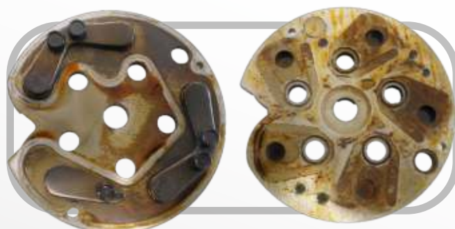
Clear sign of overheating on valve plates
