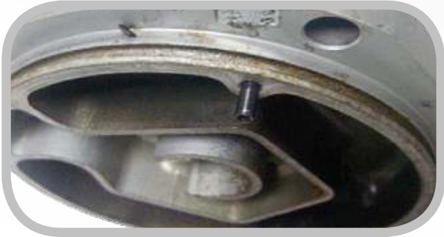
Oring groove is dirty
