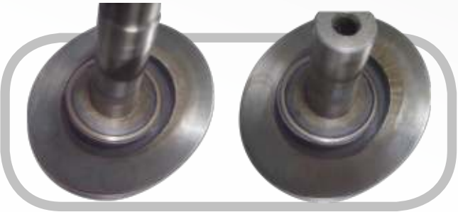
Front and rear surfaces of swashplate
