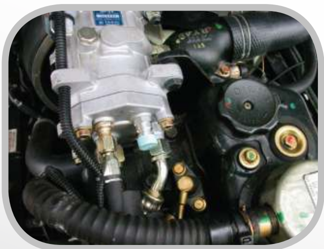
Rear view with horizontal refrigerant hose connections, plus oil return line fitted in place of suction service fitting to rear cap.
