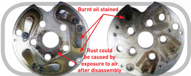
Rear discharge valve plate assembly (front & rear)
