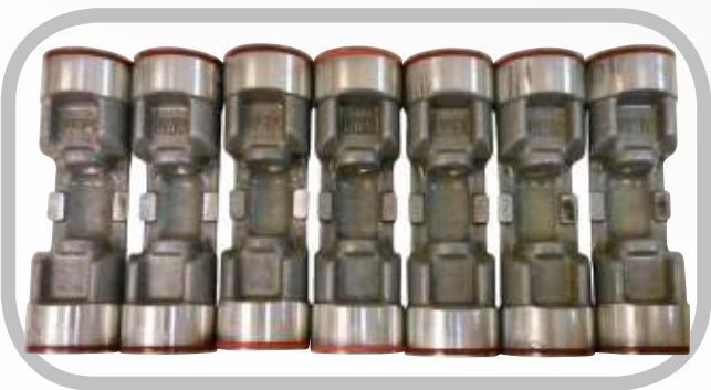
Pistons from the compressor
